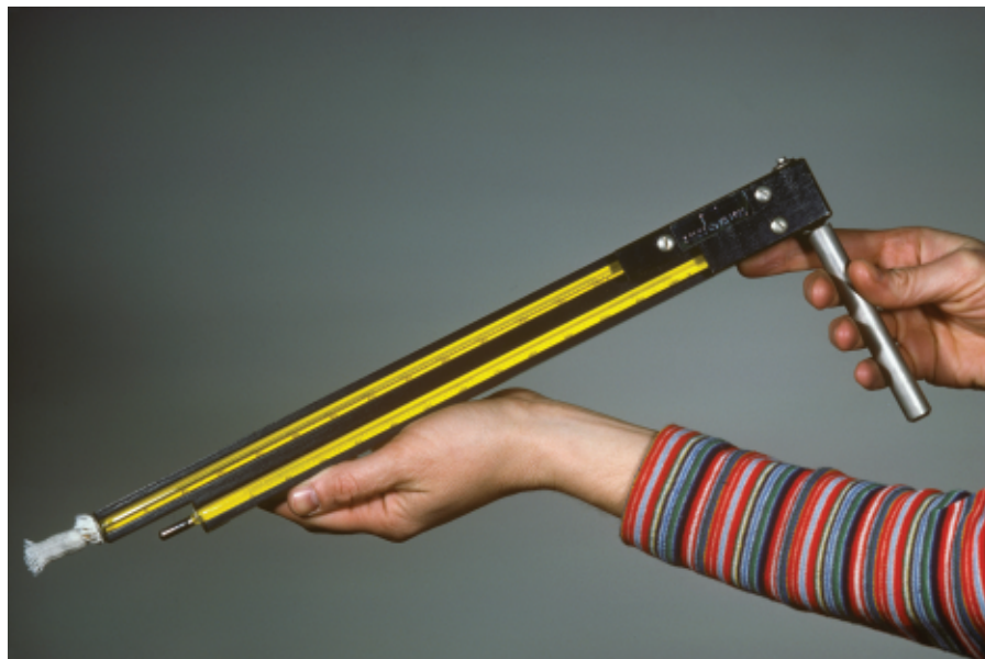
Figure 4 A psychrometer shows differences between wet-bulb and dry-bulb temperatures that can be used to determine relative humidity.
