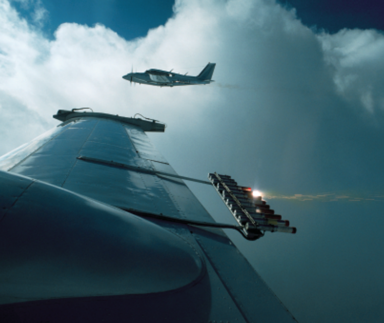
Figure 5 Special equipment attached to the wings of cloud-seeding planes releases freezing nuclei into clouds. Meteorologists hope that cloud seeding will induce rain to fall on drought-stricken areas.
